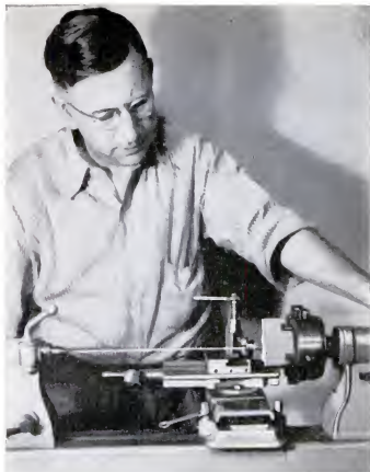
Using the indicator to center a punch mark in an irregularly shaped casting prior to boring
